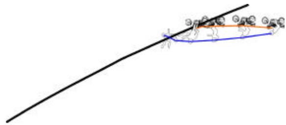
Figure 11. Trajectories determined from the overhead-view cameras of the motorcycle and the dummy before and after impacting the steel guard rail (Figure 10)
