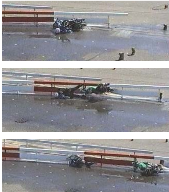
Figure 17. Full-scale crash test where the sliding motorcycle impacted the modified steel guard rail system
